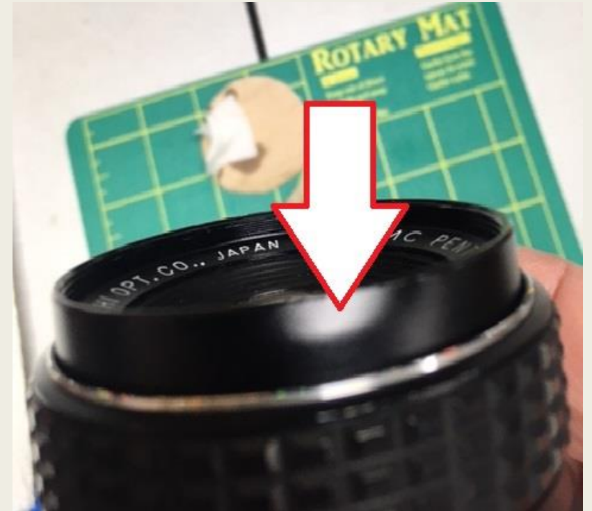
Bent filter threads: impossible to screw on a lens filter
